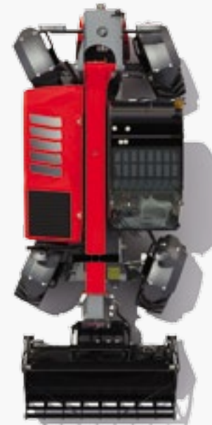
Four-wheel steering mode – for minimum turning circles.
