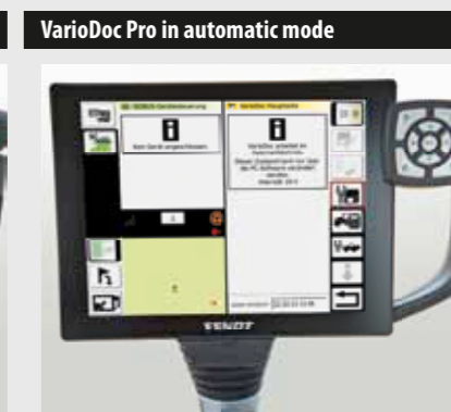
Modern field database software allows VarioDoc to start logging the relevant data automatically. Afterwards, the software assigns the data to the different fields based on the logged position data. Maximum convenience, because you get the data without any effort.
