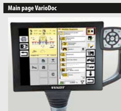
Different kinds of information are displayed on the main VarioDoc page. These include the name of the job, field name and area, crop, company and customer as well as the operating materials used. Using the virtual keyboard in the right-hand bar, recording can be started, for example.
