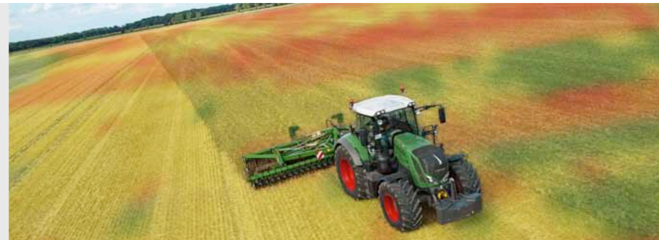
VarioDoc Pro delivers accurate position data for your field record. Machine data, such as engine speed, fuel consumption or PTO speed, can be recorded at each position. Depending on the version you have, you can visualise the work that has been performed on your PC graphically, for example, with the aid of maps, which show the relative fuel consumption or the pulling power required. This is a significant advantage over non-integrated retrofit systems.
