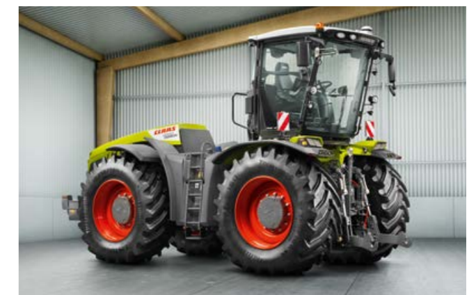
The TRAC VC has the most convenient reverse-drive system on the market. Its cab can be rotated through 180° in less than 30 seconds.
