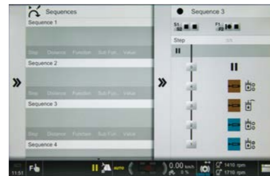
You can enter up to four sequences for four different implements or jobs
