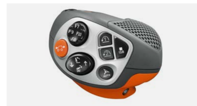
Activate the sequence using the F buttons on the CMOTION control lever
