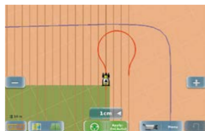
With AUTO TURN the tractor turns automatically at the headland
