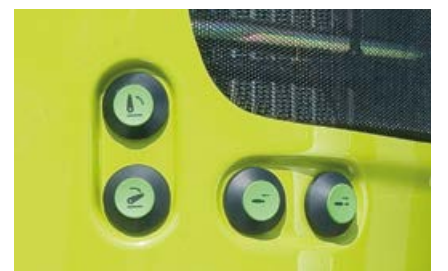
The front linkage and one spool valve are easily operated by push buttons at the front of the bonnet
