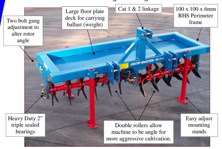
This versatile implement will aerate, cultivate and renovate your soils. The tines have a slight twist in them which cracks the ground in a sideways and downwards motion. This allows water, air and nutrients to move readily through the soil profile making them more available for plant roots.
