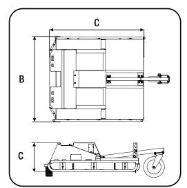
The Slasher is a slashing attachment for skid steer loaders which can be used for the effective cutting and clearing of grass and low ground shrubbery.
