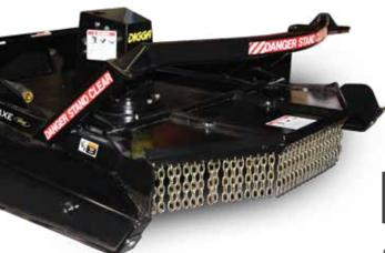
Digga's new heavy duty 72" brush & tree cutter is the ultimate attachment for clearing & shredding thick bush & scrub. Working in conjunction with the heavy duty push bar, the front hood opens up exposing the 3⁄4" blades past the guards, enabling close up axe-like cuts to remove trees up to 7" (180mm) in diameter.
