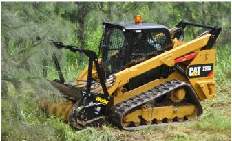
The Magnum Mulcher is the perfect for clearing firebreaks, land clearing, maintenance of park or forestry trails, utility line clearing, vegetation management and re-mediation. Suited to High Flow Skid Steer Loaders & Excavators up to 20 tonne the Mulcher is ideal for grinding small and large material, trees or brush up to 8" in diameter.
