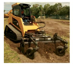
The new Fully Hydraulic 72" and 90" Digga Power Rakes grades, levels, rakes and removes debris, pulverizing and preparing the ground for a new seedbed or turf. De-thatch or remove old lawns and weeds... All with one tool.
