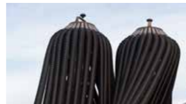
External distributor heads with straight hose runs for good seed flow
