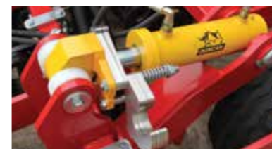
Depth adjustment on rams
