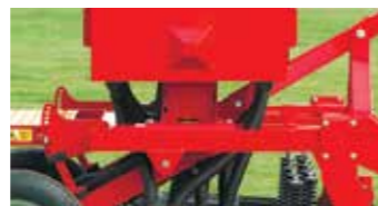
Guards on both ends of the drill to avoid snagging vines/trees
