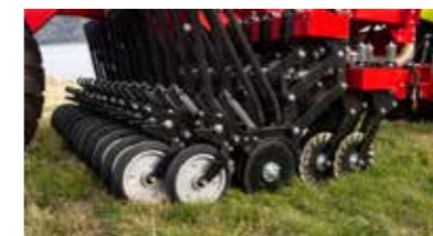
Opening Turbo Tilth disc, double discs on parallelogram & press wheels
