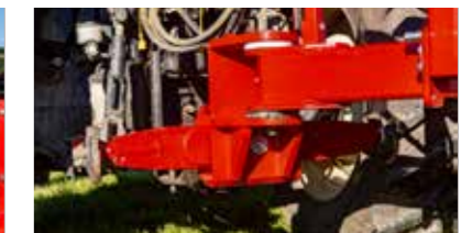
2 point hitch tow coupling
